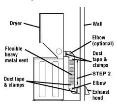
STEP 3. Add 10 inches to the measurement for each bend in the vent.
